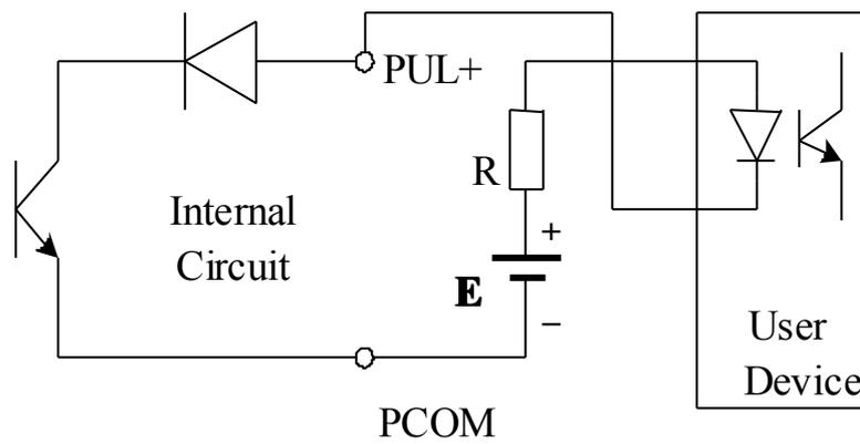
Fig. 14(e) Connection with photo-coupler (e.g. PLC)
