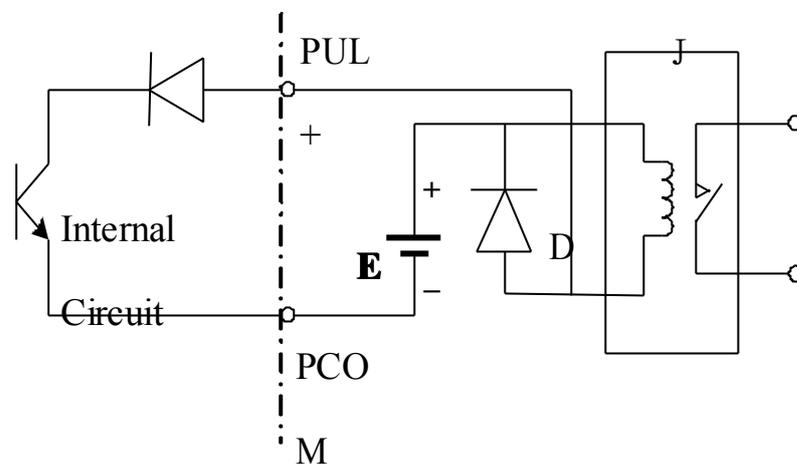
Fig.14 (f) Connection with relay (e.g. PLC)
