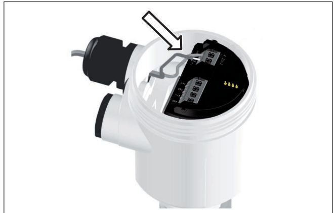
Fig. 21: Connection steps 5 and 6 - Single chamber housing
